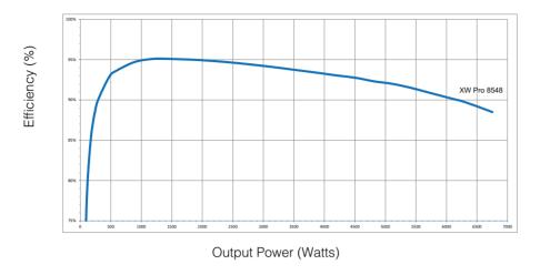
Figure A-3 Inverting Efficiency (Typical)
